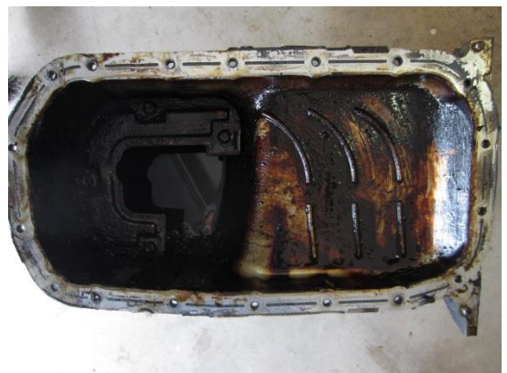
Figure 1 - Sludge Build Up
