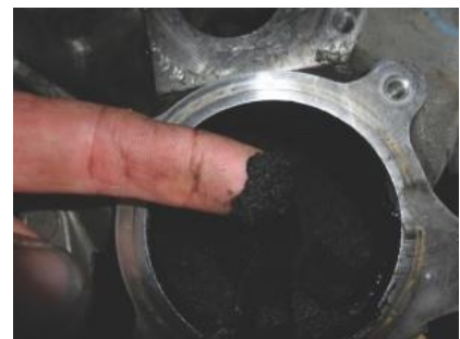
Figure 2- Soot Build Up
